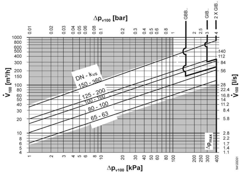
$\Delta p_{max}$  = Maximum permissible differential pressure across the valve, valid for the entire actuating range of the motorized valve.
