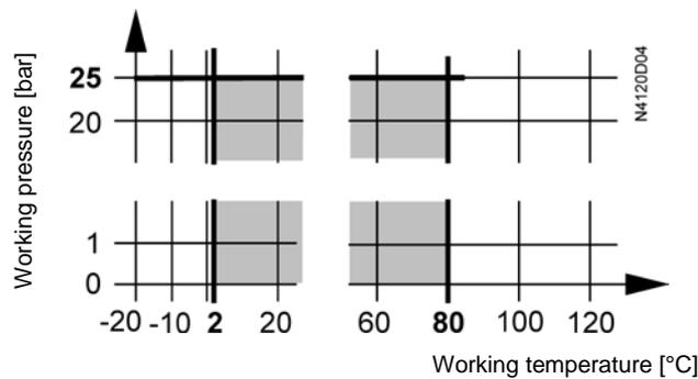
**Working pressure and medium temperature as per ISO 7005**
