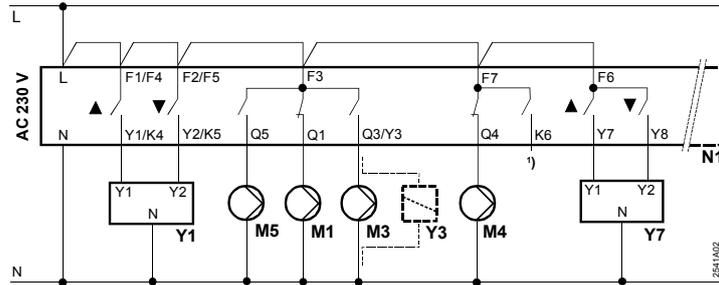
Basic connections for plant types with 2-position control (boiler with a 2-stage burner)
