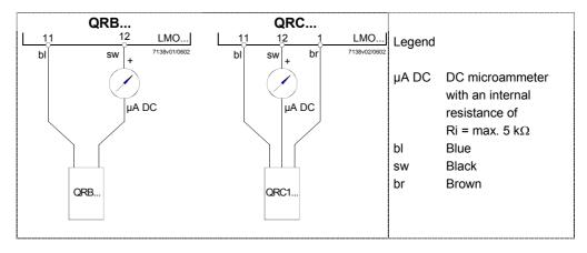
As an alternative to detector current measurement, the diagnostic tool OCI400 / ACS400 can be used. In that case, connection of the DC microammeter is not required.
