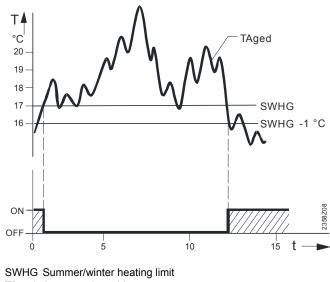
TAged Attenuated outside temperature T Temperature
