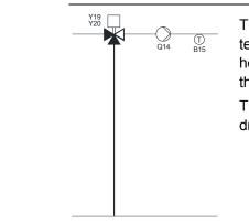
The primary controller allows lower or higher flow temperatures by mixing to obtain flow temperatures for heating/cooling zones with setpoints higher or lower than those of the common flow.
