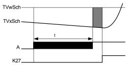
TVxSch Actual value of common flow temperature TVwSch Setpoint of common flow temperature А Request Release output K27 K27 Locking time
