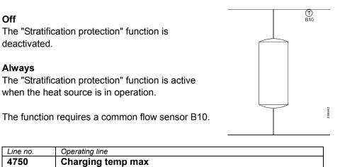
Solar energy charges the buffer storage tank until the set maximum charging temperature is reached.
