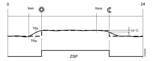
Xein Forward shift of switch-on time
