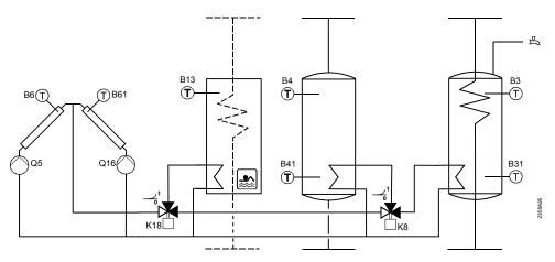
If sufficient solar energy is available, the solar plant can heat the swimming pool, the DHW storage tank and the buffer storage tank. Priorities for heating or charging the different storage tanks can be selected. The pumps can be speed-controlled. Protection of the plant is ensured by a "Frost protection" and an "Overtemperature protection" function.
