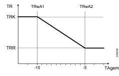
TRwA1Reduced setp increase endTRwA2Reduced setp increase startTRKComfort setpointTRRReduced setpointTAgemComposite outside temperature
