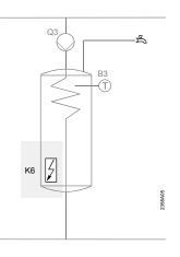
If DHW charging is interrupted because the heat pump exceeded the permissible number of charging attempts (line 2893), the electric immersion heater (K6) – if installed – completes the charging process.
