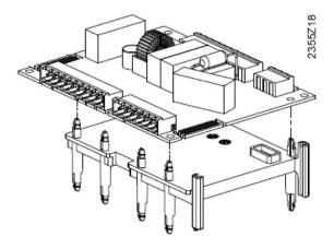
Then, plug the spacer plate together with the I/O module onto the basic unit.
