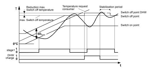
Behavior of Q9 with buffer storage tank at the maximum switch-off temperature If, due to "Switch-off temp max" (line 2844), the heat pump had to shut down and a new start is made, condenser pump Q9 is put into operation first and then the compressor, whenever the following criteria are satisfied:
