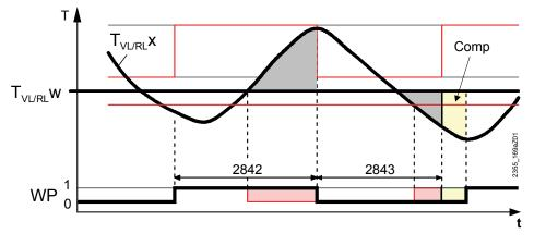
$\begin{array}{ll} T_{VL/RL}x & \mbox{Actual value of flow or return temperature} \\ T_{VL/RL}w & \mbox{Flow or return temperature setpoint} \\ 2842 & \mbox{Compressor run time min} \\ 2843 & \mbox{Compressor off time min} \\ WP & \mbox{Heat pump switching state: 0 = off, 1 = on} \\ \mbox{Comp} & \mbox{Compensation of surplus heat resulting from running time} \\ \end{array}$
