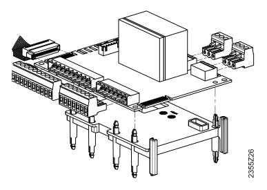
Then, plug the spacer plate together with the I/O module onto the basic unit.
