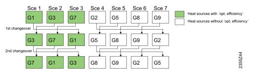
Sce: Heat source Gx: Device address Setting the heat source sequence exclusion is only used in connection with the activated heat source sequence (line 3540).
