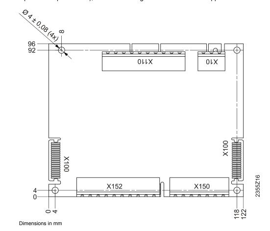
Dimensions and drilling plan
