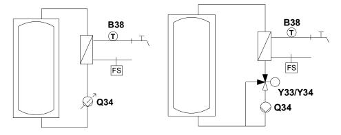
When the DHW flow switch (FS) detects flow, sensor B38 provides control to the nominal setpoint (line 1610).
