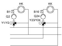
Cooling and heating circuit draw their cooling energy/heat from separate common flows.
