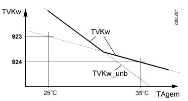
TVKwFlow temperature setpoint for cooling (with minimum limitation)TVKw\_unbFlow temperature setpoint for cooling (without minimum limitation)TAgemComposite outside temperature
