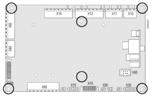
The I/O module (AVS55.196 or AVS55.199) can be fitted next to the basic unit or using a spacer - can be plugged onto the PCB of the basic unit (refer to description of the AVS55.196 or AVS55.199).
