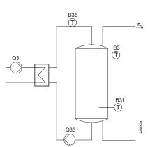
Intermediate circuit boost For charging, the flow temperature in the intermediate circuit (B36) must exceed the required DHW setpoint by the value set here because the heat exchanger is not able to transfer all energy.
