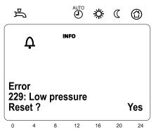
After pressing the OK button once, "Yes" is displayed flashing. Pressing the OK button a second time confirms the "Yes" and resets the error.
