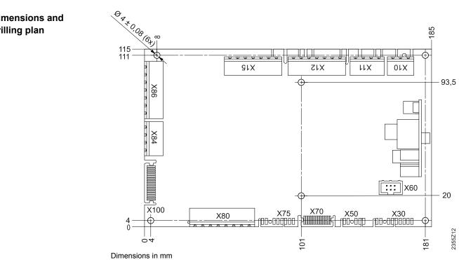
**Dimensions and** drilling plan
