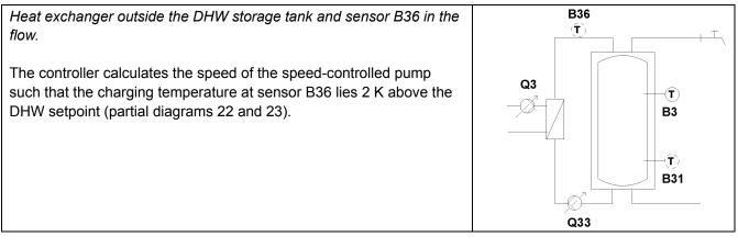
Heat exchanger outside the storage tank, with primary controller.
