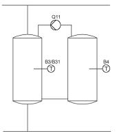
If the temperature level of the buffer storage tank is high enough, the DHW storage tank can be charged by the buffer storage tank.
