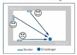
Tip Avoid RF transmission along wall surfaces (e.g. in a long hallway as well).
