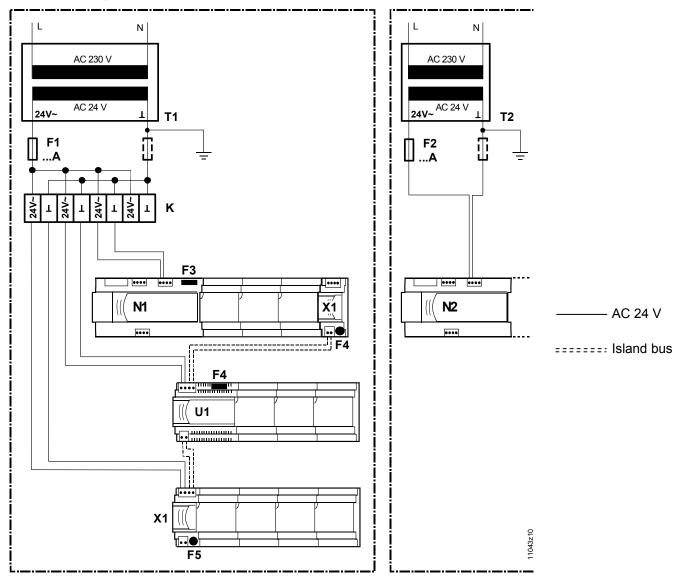
Key T, T2 Safety transformer AC 230 V / AC 24 V as per EN 61 558.
