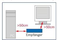
The distance of the EnOcean receiver to other high frequency transmitters should be at least 50 cm.
