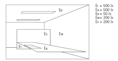
Fig.: Examples for brightness on various locations in a typical office (desk EA = 500 lx)
