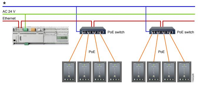
\* Supply voltage and power depend on the type of PoE switch used and the number of connected room operator units.
