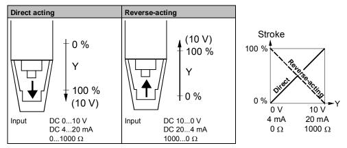
The mechanical spring-return function is not affected by the direction of operation
